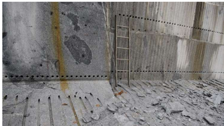
Figure 3.- Quarry in a white granitic massive rock formation exploited for dimension stones: boreholes are closely spaced for the use of cutting methods (in this case, detonating cord). Credits C. Oggeri, Northern Alps, Italy.
