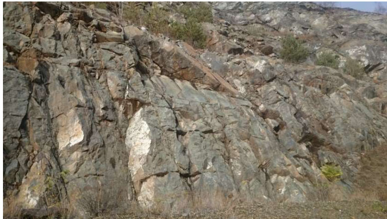
Figure 2. Blasting along the bench in a blocky quarry of peridotite (hard rock): spacing between joints: 0.5–3 m. Residual vertical blast holes are partially visible; geo-structural pattern strongly affects the result of the contour blasting (credits C. Oggeri, open pit in Western Alpine range, Italy).
