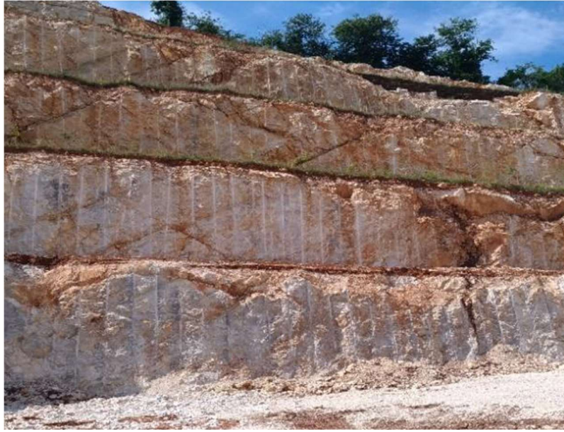
Figure 4. Quarry face in weathered limestone with evident traces of boreholes (good HCF) along the benches during the exploitation of aggregates; three largely spaced joint systems form the rock mass. (Eastern Alpine range, Italy)
