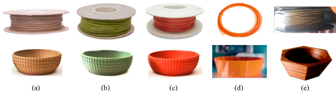
Figure 2. Thermoplastic bio-composite filaments: (a) HEMP, (b) WEED, (c) TOMATO, (d) CAROB, and (e) PRUNED.
