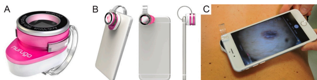
Figure 2. (A) Nurugo TM Derma; (B) Nurugo TM Derma attached to the smartphone; (C) Example of smartphone microscope applied to skin.
