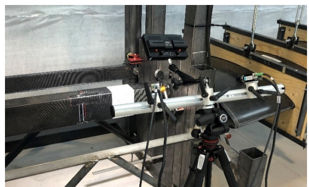
Figure 10: Test area after superficial treatment and during image acquisition.
