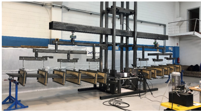
Figure 2: Experimental set-up of the wing used for the static response analysis.
