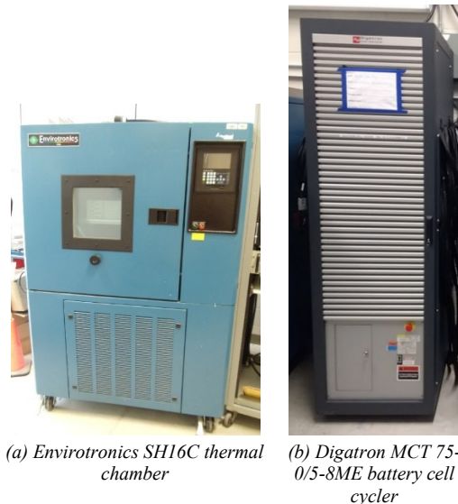
Fig. 7. Battery test equipment for ageing test
