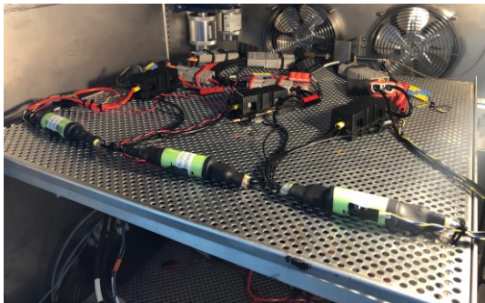
Fig. 6. Tested cells mounted in the thermal chamber.
