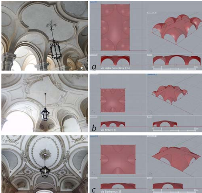
Fig. 5. Parametric models of Planterian vaults in Turin. Synoptic representation of selected cases by the parametric model: plan, elevations and perspective views. (a) Palazzo Saluzzo Paesana, (b) Palazzo Villanis, (c) Palazzo Perucca della Rocchetta. Models: Marco Vitali (From Vitali, 2017)
