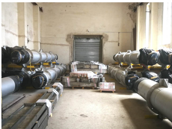
Fig. 2 The central modules of the column stored at Carbosulcis S.p.A., Nuraxi-Figus site, ready for installation.
