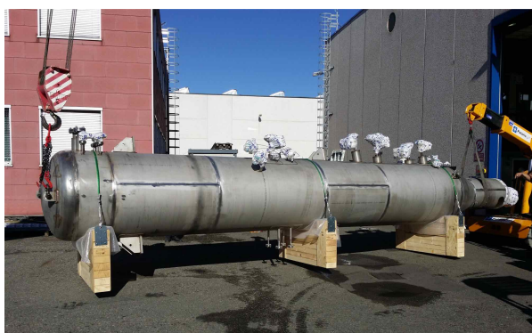
Fig. 3 The top module of the column.
