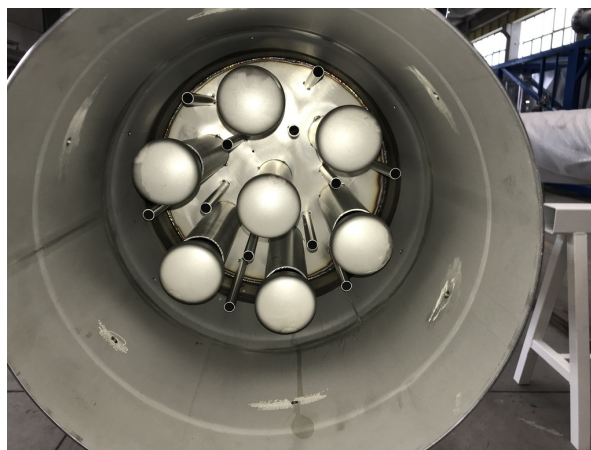
Fig. 5 A view from above of a liquid distributor.
