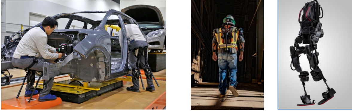
Figure 7. Left: Chairless exoskeleton (H-CEX) (Image source Hyundai Inc.); Middle: Back support exosuit; Right: Whole-body suit (Image source: EksoBionics).
