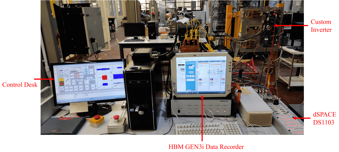
Figure 2.2: Experimental Setup with the custom built inverter, dSPACE DS1103 control platform and HBM GEN 3i data recorder.
