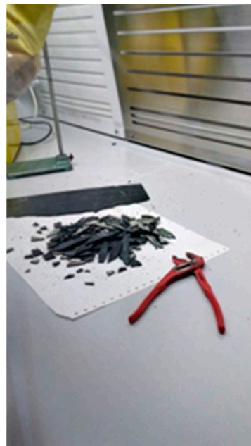
Figure 9. Multigrip plier breakage test.
