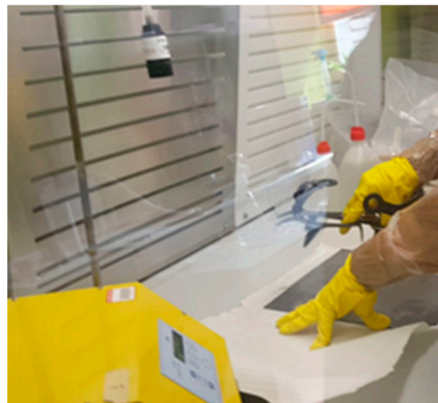
Figure 10. Vinyl tile crampon test inside the confined hood.
