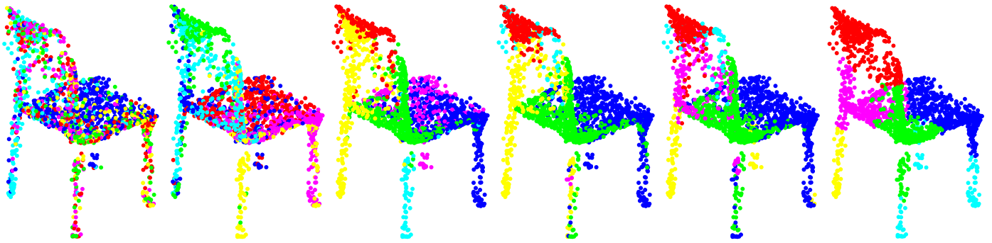
Fig. 8: No upsampling: k -means clustering of features of intermediate layers, highlighted onto the output point cloud (leftmost: output of dense layer, rightmost: output point cloud). Notice how layer features generate clusters that are progressively more localized in the output geometry.
