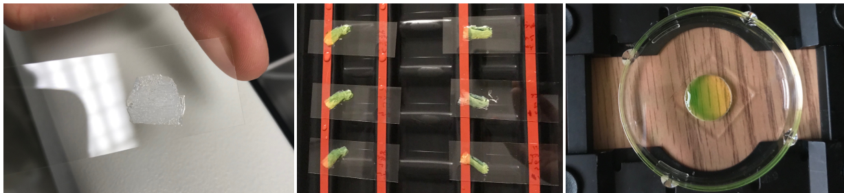
Fig. 4: An MCL section (left), a set of stained MCL sections, and a solution of 3 kDa FITC-dextran and PBS, placed on a glass bottom dish to minimise fluid drift during the FRAP experiments.
