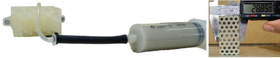
Figure 5.17: Sample of Calcium-Bentonite-Alginate manufactured with a honeycomb structure and applied with a dip molding technique on a conventional packed heat exchanger.
