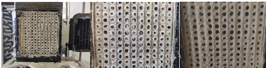
Figure 5.20: The picture in the left and in the middle are showing the deformation resulting from the curing operation at 85°C for 12 hours. The initial honeycomb geometry of the air channels is definitively lost. On the right the different appearance once exposed to air, the material absorb moisture.
