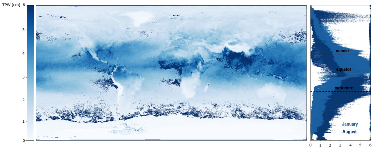
1339 Figure 4.2: TPW distribution from data provided by MODIS instrument onboard of Terra satellite (parameter MOD05_L2). Data depicts 1340 the average distribution during August (2019). Water vapor are determined with errors typically in the range between 5 and 10 percent 1341 [192][193]. On the right the spectral distribution of the map over the latitude for the average day of January and August 2019. The 1342 interesting aspect is the seasonal movement of the climatic equator . 1343
