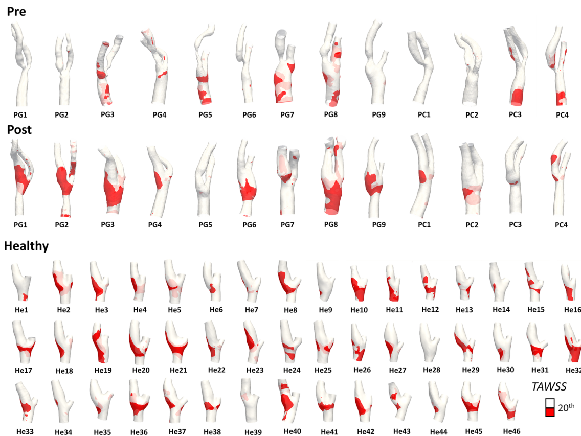
FIGURE 7. Luminal surface area exposed to low Time-Averaged Wall Shear Stress (TAWSS) as expressed by the Low Shear Area (LSA), in pre-CEA (Pre), post-CEA (Post) and healthy cohorts. The LSA in pre-CEA and post-CEA cohorts is extended beyond the bifurcation region (delimited by sections CCA3-ICA5-ECA2) to include in the pre-CEA models possible distal stenoses. Red areas represent TAWSS value below the 20th percentile of the pooled TAWSS distribution of the healthy models in the bifurcation region.
