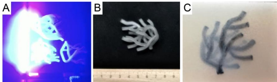
Figure 4. Phantom manufacturing. (A) 3D printing process; (B) final model; (C) final phantom in agar.
