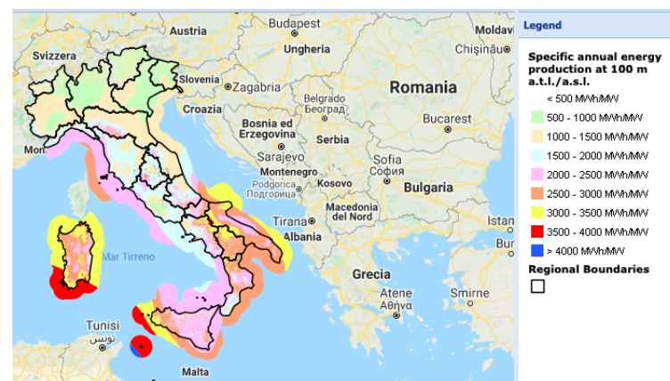
Figure 11. Specific producibility of onshore wind at 100 m (above ground level) and offshore wind at 100 m (above sea level) [57].
