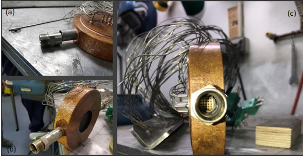
217 218 Figure 3 - Details of the RRs Mock-up welding to the connection pipes of the solar furnace: (a) before welding, 219 (b) after welding, (c) view of the inside of the two connected pipes. 220
