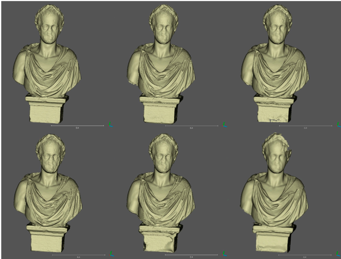
Figure 11. Untextured meshes of the stone bust from dataset 6 (from left to right, and from top to bottom): F6 SR, AMP, FZA, ARP, VCM, R3D.
