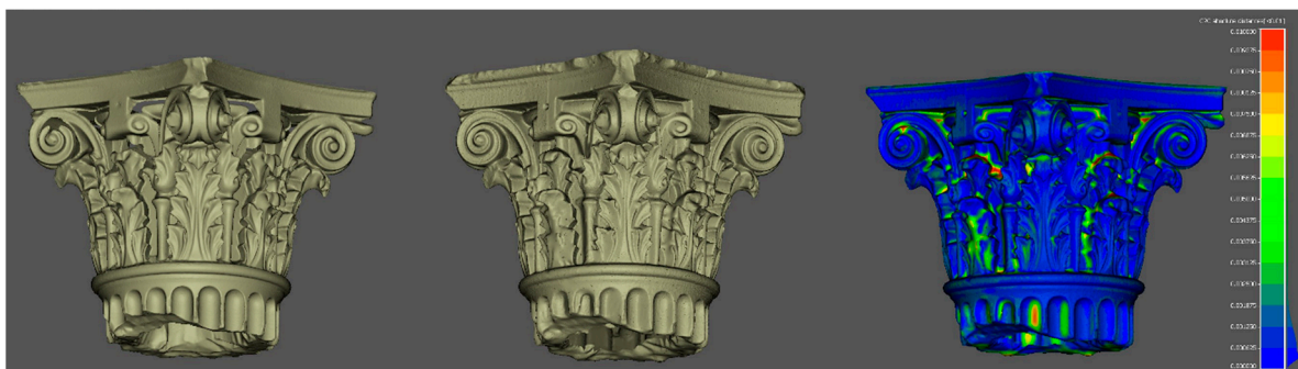
Figure 4. Scanning results. Untextured Stonex F6 SR mesh ( left ), untextured FARO Focus 3D X 330 mesh ( center ) and scalar field mapping of Hausdorff distances; maximum visualized distance: 1 cm.
