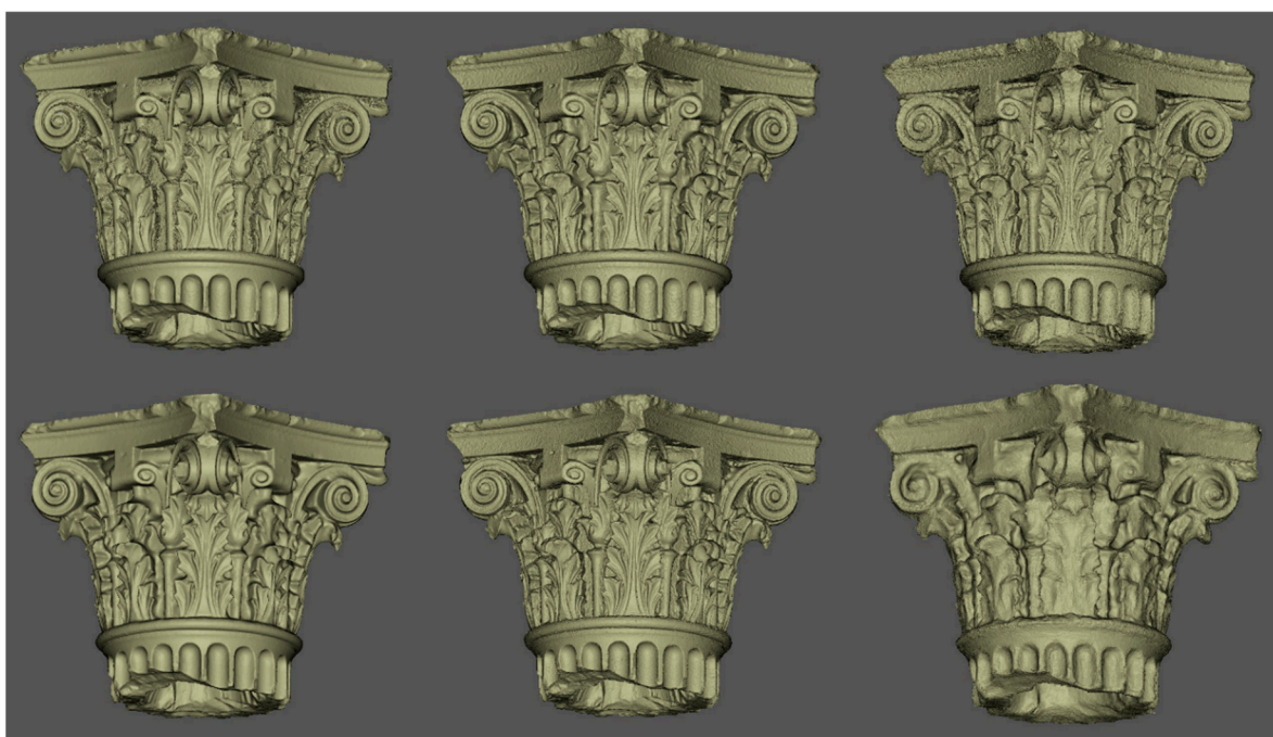
Figure 10. Untextured photogrammetric meshes of the capital replica from dataset 5, (from left to right, and from top to bottom): AMP, FZA, P4D, ARP, VCM, R3D.
