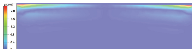
Fig. 12. Current density distribution for the unskewed rotor cage (component in the lamination plane – Fig. 11 on the right – in locked rotor condition).
