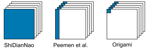
FIGURE 39. Different solutions [129], [131] [130] to spatially unroll the computations in an output stationary dataflow.
