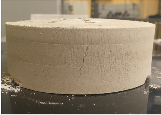
Fig. 10. Small crack developing on the side of the 110 mm sample [14]
