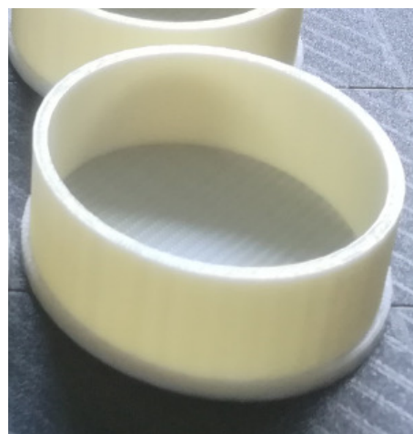
Fig. 1. Mould for suction controlled oedometer test [8].
