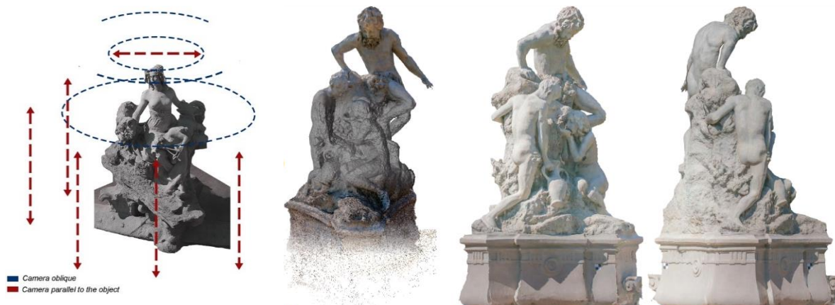
Figure 4. Flight schemes of the DJI Spark on the sculptural groups (left) and some examples of the acquired images (right).
