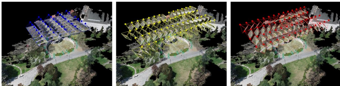
Figure 2. The UAVs flight plans: Nadiral (left), oblique (centre), oblique flight with PoI (right).
