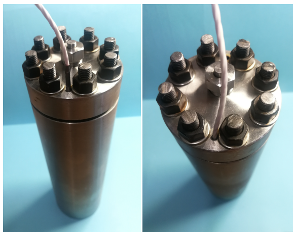
Figure 8.12: Thermometer housings into the pressure vessel walls.
