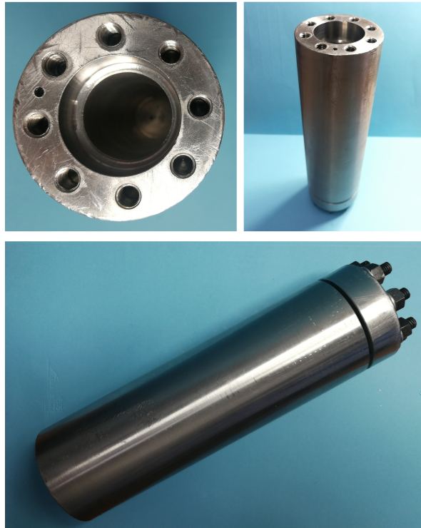
Figure 8.4: Stainless steel pressure vessel used to carry out speed of sound measurements at high pressure.
