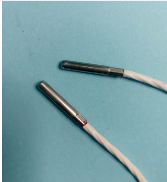
Figure 8.9: Picture of the two platinum resistance thermometers used to measure the system temperature.
