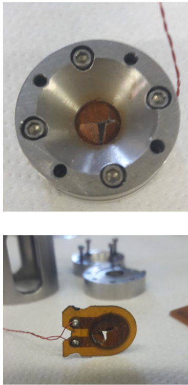
Figure 8.7: Picture of a broken piezo-ceramic transducer, after a thermal shock.
