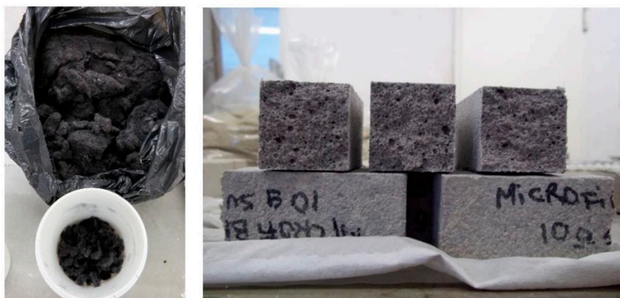
Figure 3. ReCash Plaster (Recycled Cashmere for Plaster): from textile waste to experimental specimens. On the left, wool and cashmere dust; on the right, pre-mixed plaster obtained by replacing glass fibres with textile waste.
