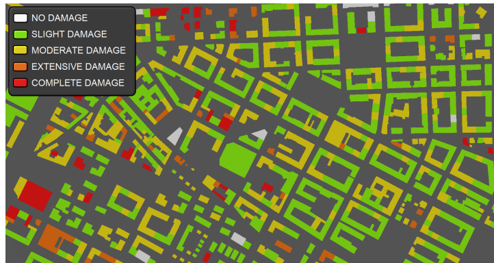
Figure 4: Detail of the IdealCity plan with damage assessment.
