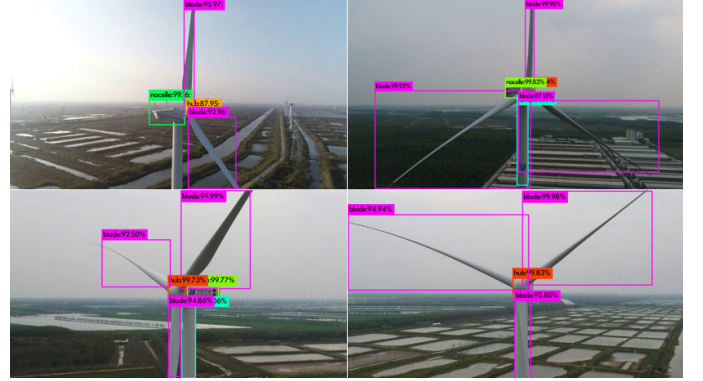
Fig. 8. Detection results by YOLOv3 network of wind turbine with different blade rotation angle and environment conditions: nacelle (green bounding box), hub (orange bounding box), blades (magenta bounding boxes), and tower (cyan bounding box).
