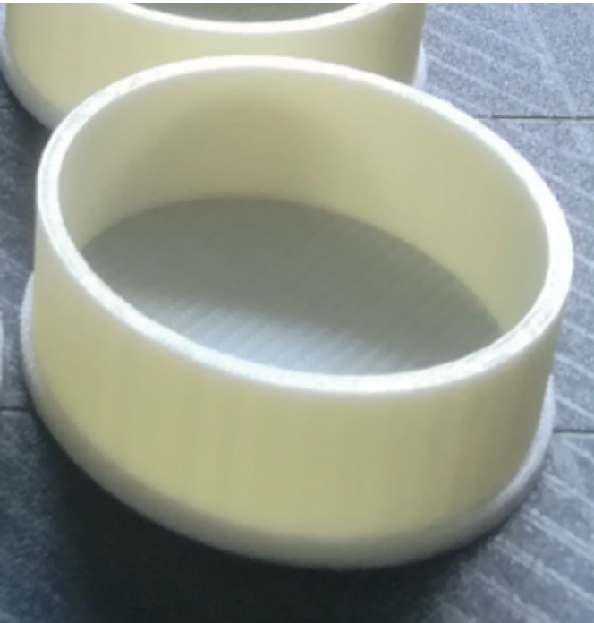
Fig. 1. Molds for the preparation of specimens for oedometer testing (left, internal diameter 50.5 mm and height 20 mm) and for triaxial tests (right, internal diameter 38.1 mm and height 76.2 mm )
