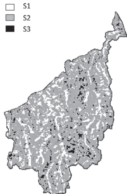
Fig. 3. Map of susceptibility to shallow landslides for the Cellio Municipality (VC). Classes of susceptibility: very low (S1), low/moderate (S2) and high (S3)
