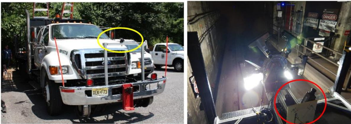
Figure 9. Camera Scanning Rail Truck with a single camera (left), and Cameras Scanning the Tunnel with two IR cameras (right)
