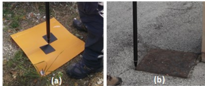
Figure 4.12. Artificial GCP marker (a), and natural GCP marker (b).
