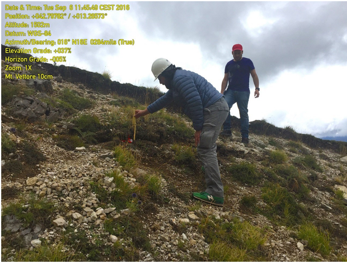
Figure 2.19c. Mt. Vettore fault Site 1 at a WGS84 ellipsoid elevation of 1502 m. The normal fault displacement at this site was 10 cm down toward the west (Latitude and Longitude are annotated on the image).
