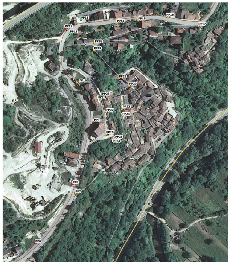
Figure 4.13. Position of the GCPs in Pescara del Tronto (red indicated artificial marker, green indicates natural marker).
