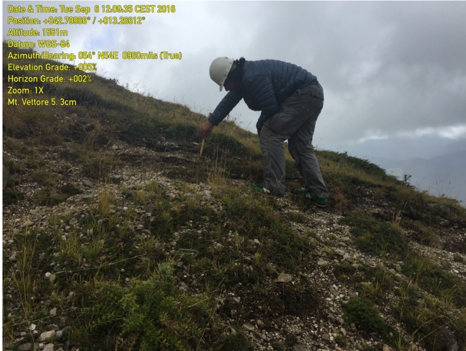
Figure 2.19g. Mt. Vettore fault Site 5 at a WGS84 ellipsoid elevation of 1561 m. The normal fault displacement at this site was 3 cm down toward the west (Latitude and Longitude are annotated on the image).
