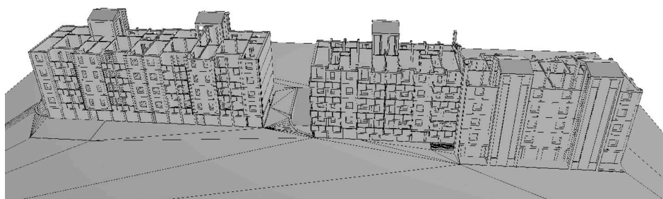
Figure 4. Example of Savigliano model converted to CityGML. Each object is converted to GenericCityObject , with lod4Geometry .
