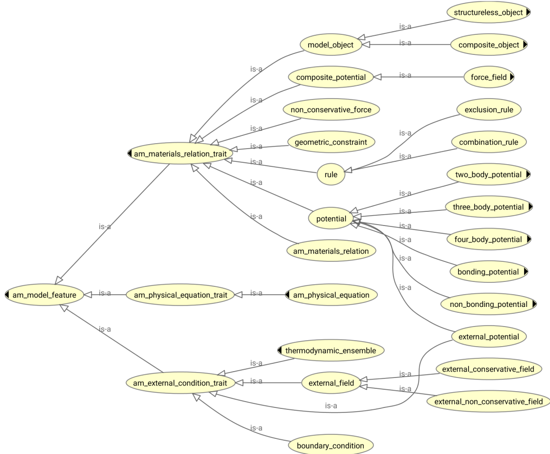
Figure 1: VISO class am_model_feature and its subclasses. This figure and similar ones in the present article have been generated using OWLViz. 82
