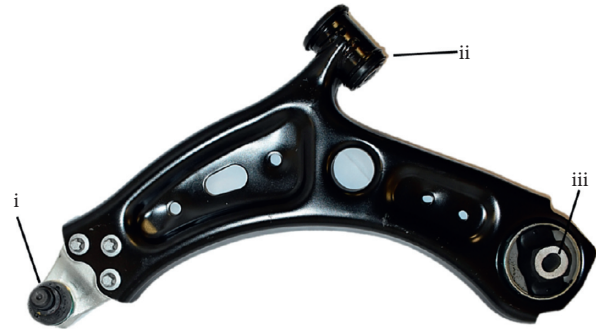
FIGURE 1: Lower control arm: the complete assembly is composed of the lower ball joint (i), front bushing (ii), and rear bushing (iii).
