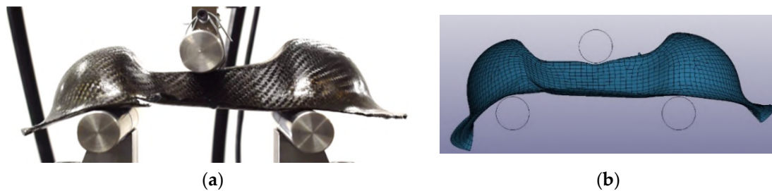
Figure 33. Experimental–FEA visual comparison during the three-point bending test on the CF/PA66 Double Dome: experimental test (a) and virtual simulation (b).
