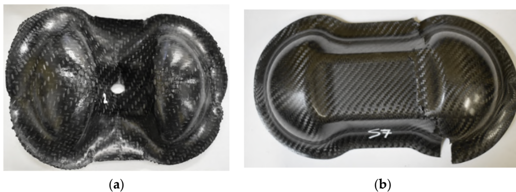
Figure 31. Double Dome specimens in GF/PP (a) and CF/EP-Solvay (b) after the bending test.
