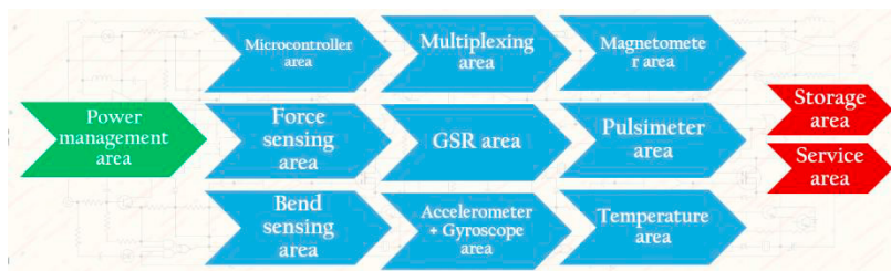
Figure 1. Functional areas of the electronic evaluation board.
