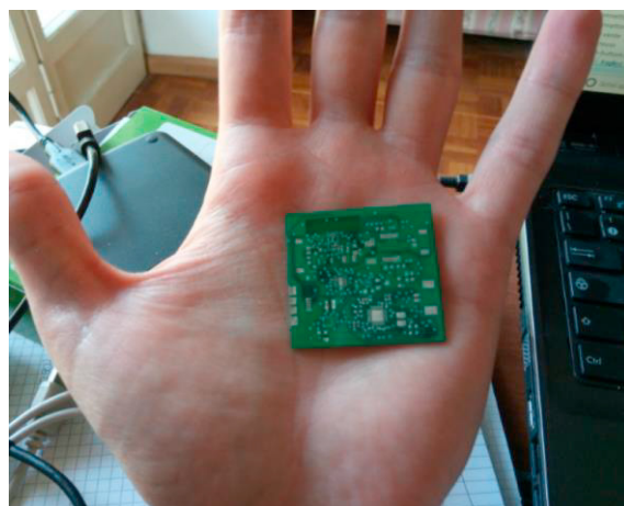
Figure 4. Final layout configuration and image of the miniaturized control circuit.
