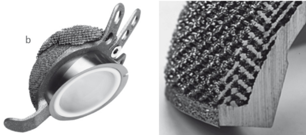
Figure 1: Hip prosthesis and trabecular lattice surface in titanium alloy [1].
