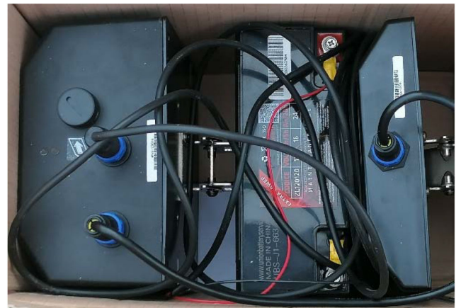
Fig. 1 Photo of BT and WF scanners used during the on-field tests composed by the scanner, the battery and the antenna
