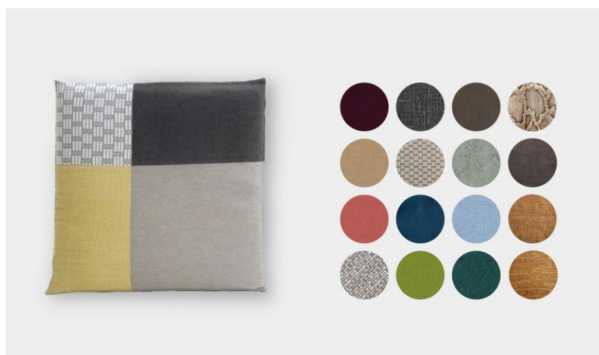
Figure 5 On the left, one of the prototypes of insulation acoustic screen manufactured within EDILTEX project. On the right, a list of available textile and leather waste samples.
