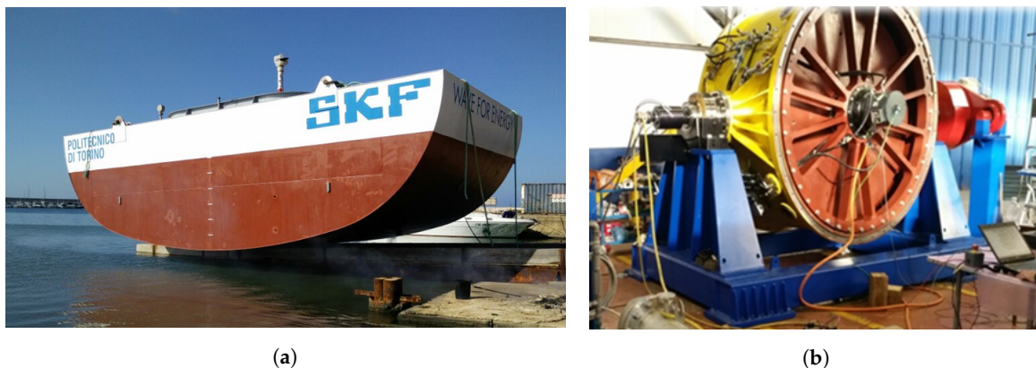
Figure 1. ISWEC device installed in Pantelleria island (Sicily, Italy): (a) ISWEC Pantelleria hull; (b) ISWEC Pantelleria gyroscope.
