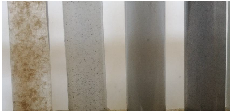
Figure 5: Dispersion of different graphene-based materials in water after adding 3 ml of calcium hydroxide solution, from left: GO, RGO, GNP-COOH, GNP.
