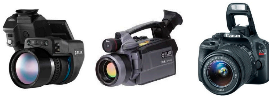
Figure 2. Instrumentation used (from left to right): FLIR T1030sc, FLIR SC660, and Canon Rebel-SL1.
