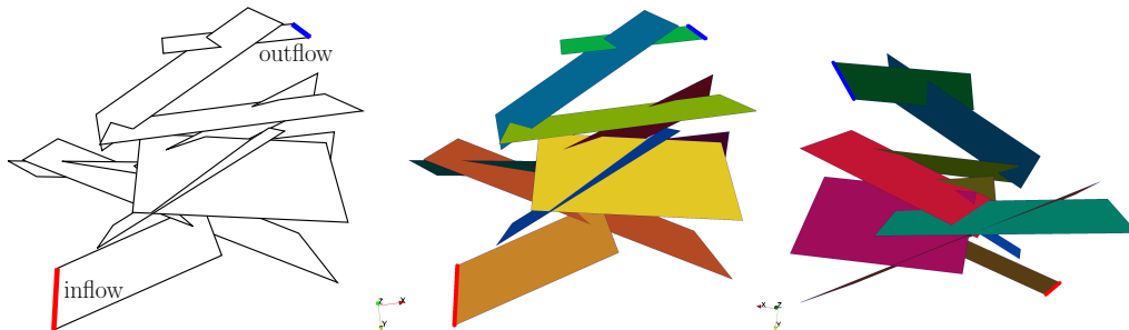
Figure 10: Geometry of Test Case 2 and two views of the network. A red line represents the inflow and a blue thick line the outflow part of the boundary, respectively.
