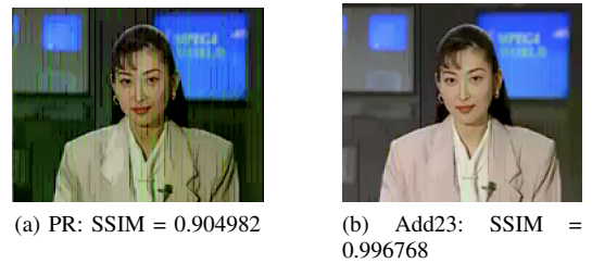
Fig. 8: Accuracy results obtained at application-level.
