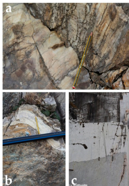
Figure 3. Outcrop appearance of the lithologies of the study area: (a) Megalodon-bearing marble, (b) Seravezza breccia, (c) contact between white and grey marbles.
