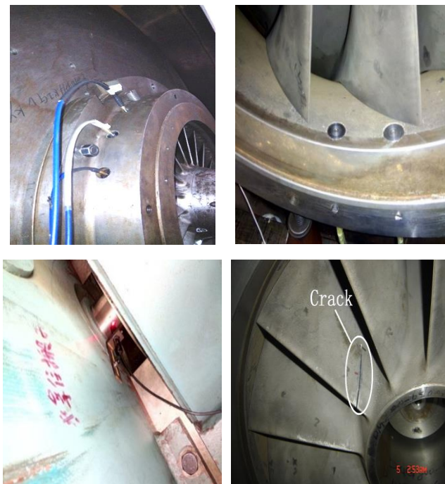
Fig. 12. The installed sensors and impeller with cracked blade.
