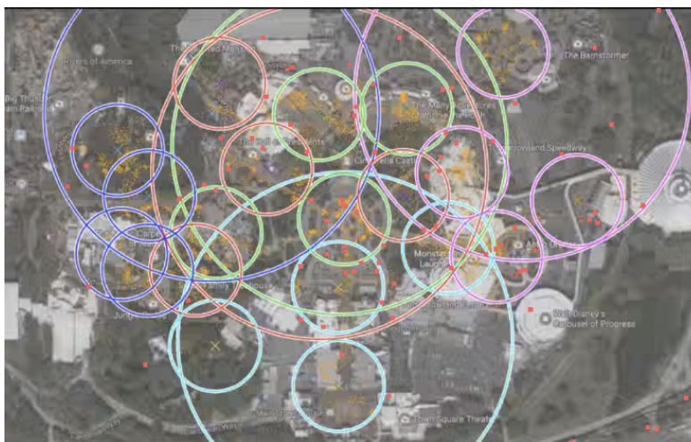
Figure 12: Real-world scenario with antennas and PoA coverages.
