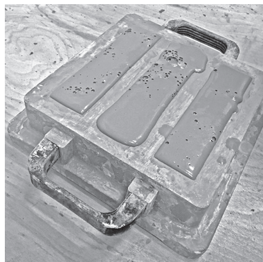
Fig. 2. Samples casted computing a bigger whole volume of material. Bubbles are clearly visible on the casting surface (on the left). Samples trimming performed by a spatula (on the right).
