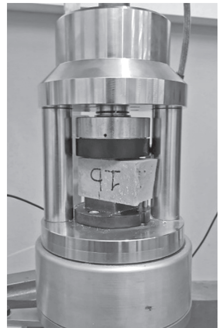
Fig. 6. Used compri-mitor according to UNI EN 196-1:16.
