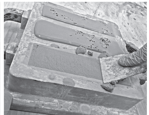
Fig. 2. Samples casted computing a bigger whole volume of material. Bubbles are clearly visible on the casting surface (on the left). Samples trimming performed by a spatula (on the right).
