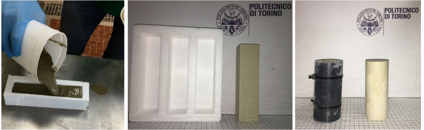
Figure 3: Casting of a prismatic sample, on the left. Example of used moulds and corresponding samples: cylindrical mould model on the right (internal diameter \phi = 52 mm, height = 130 mm) and prismatic one ( l = 40 mm, height = 160 mm) in the centre. The squares on the base background are 1 \text{ cm}^2 .
