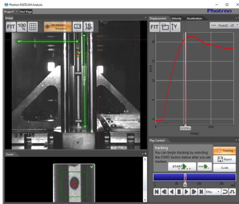
Figure 5: Tracking of the displacement of the specimen during the crush test from the high-speed video using the Photron PFA software.
