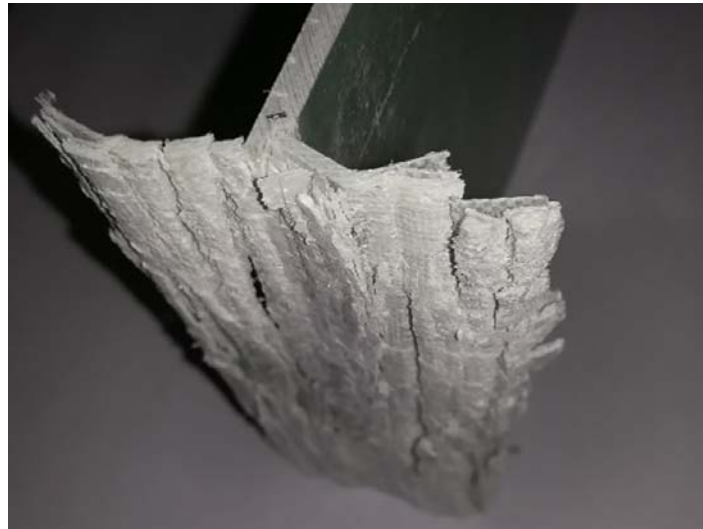
Figure 6: Detail of the crushed part of a glass fiber specimen
